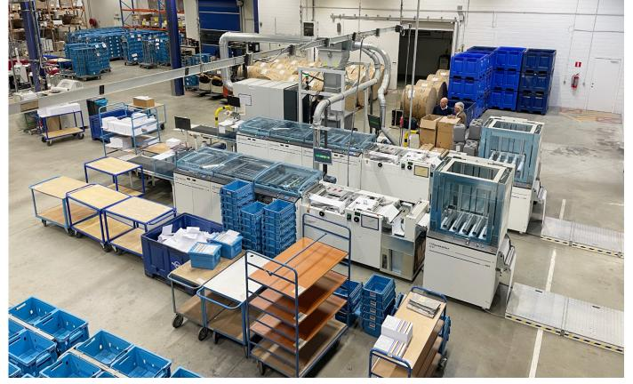
Thanks to its compact design, operation based on the proven vacuum principle and efficient filter technology, the HKU-4500 compact extraction unit could be installed right next to the CS6 finishing lines at Hunkeler AG. This in turn made it possible to keep the pipework short, with correspondingly low energy costs.
